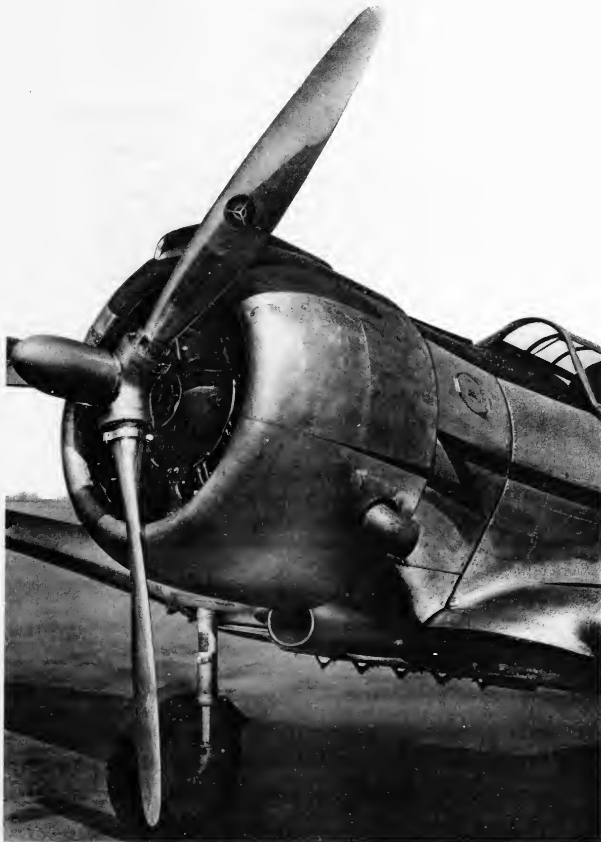
8242 - Cowling Installation - Left Side
